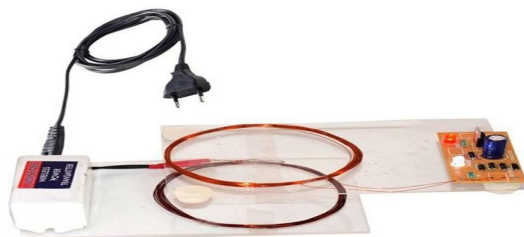
Fig. 4 Wireless power transfer
