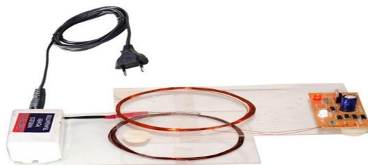
Fig. 4 Wireless power transfer
