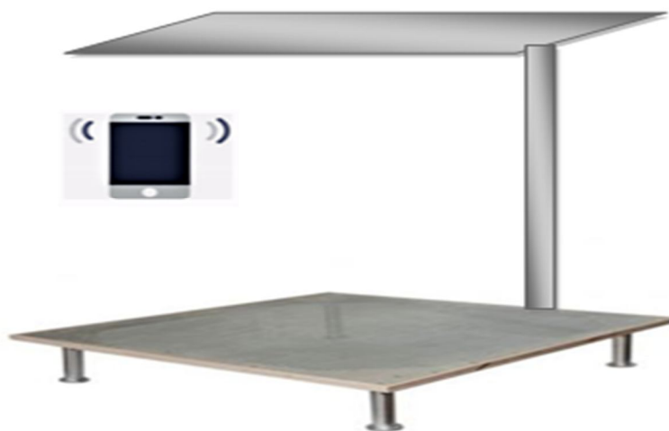
Fig. 15 Charging of mobile phone inside a closed metallic setup using ubiquitous power supply
