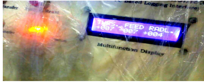
Figure 5. Digital Tool Dynamometer Showing Optimum Responses in Fx, Fy, and Fz Direction in Kg at cutting speed 180mm/min, feed rate 0.1mm, and depth of cut 0.
