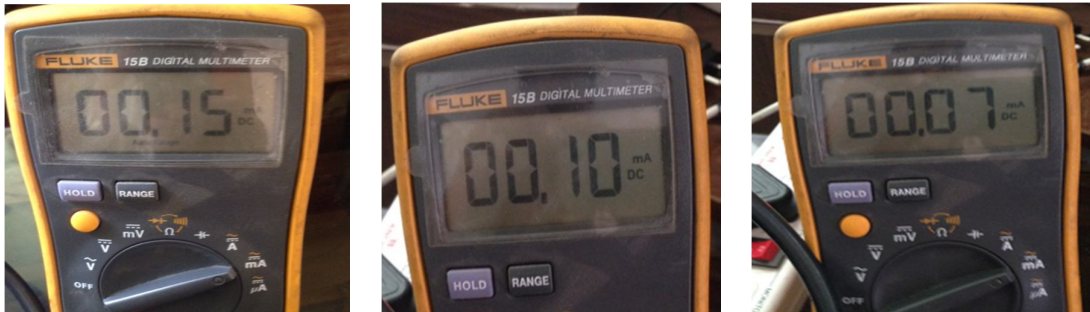
Figure-10: Power consumption results shown by multimeter in milli-amperes for the above said cases respectively
