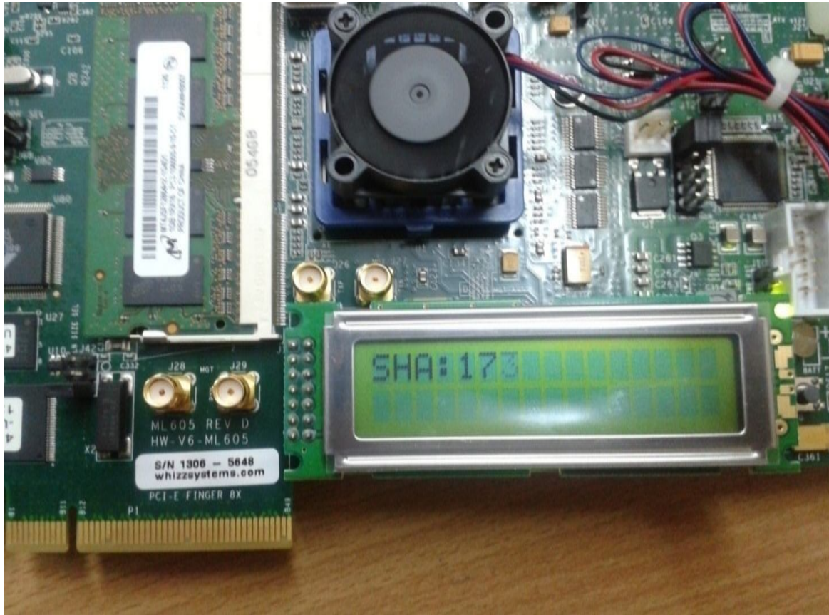
Fig. 4 FPGA implementation of SHA-512
