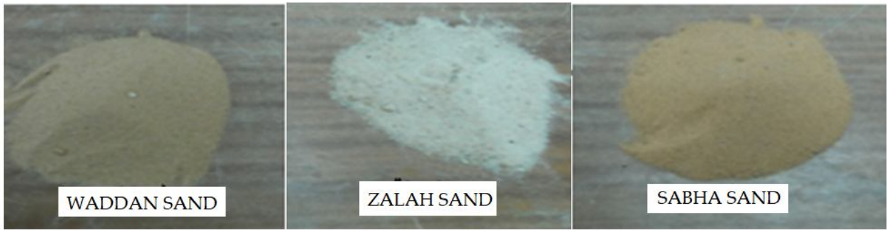
Fig 2 Types of sand used in the study
