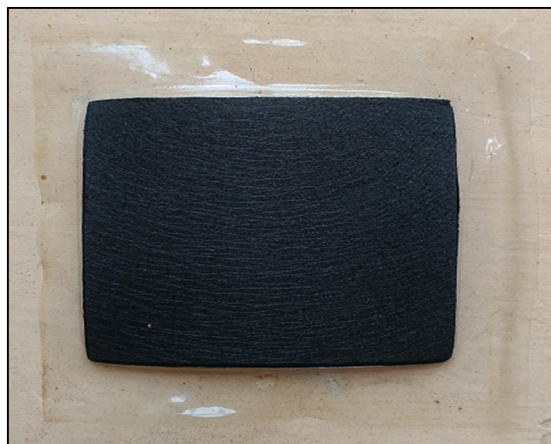
Figure 4: Membrane electrode assembly (MEA) synthesized by authors based on Decal process[24] published in literature for this review
