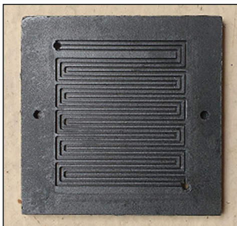
Figure 3: Flow field design on a bipolar plate [22](Serpentine flow field design)
