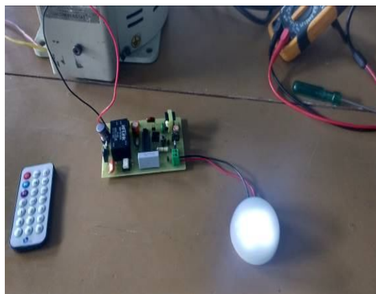
Fig. 13. LED bulb dimmed using remote control
