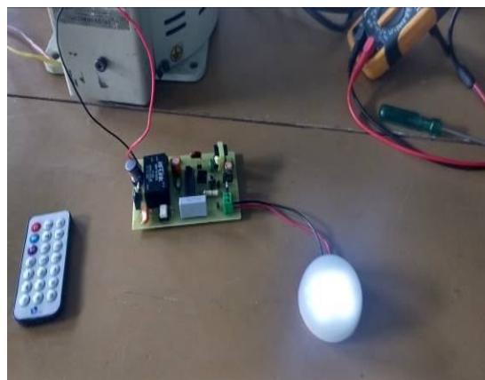
Fig. 13. LED bulb dimmed using remote control
