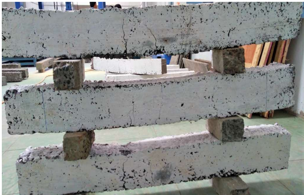
Fig 19 – Crack pattern of GPC beams with 1.5 % ,2% and 2.5% of glass fibres
