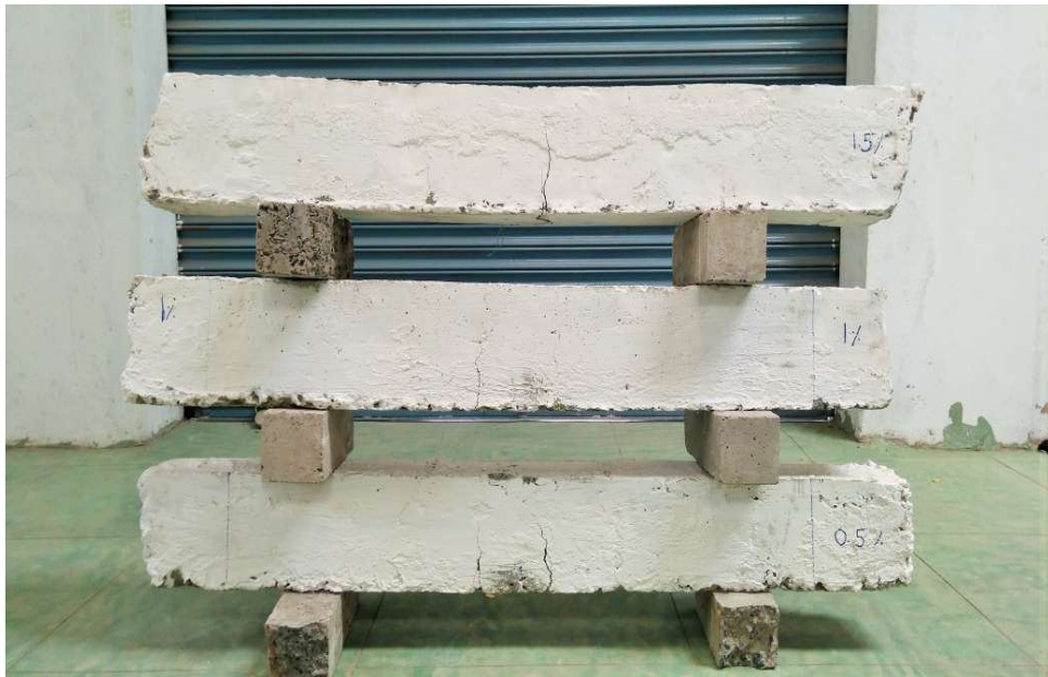
Fig 16 – Crack pattern of NVC beams with 0.5 %, 1% and 1.5% of glass fibres
