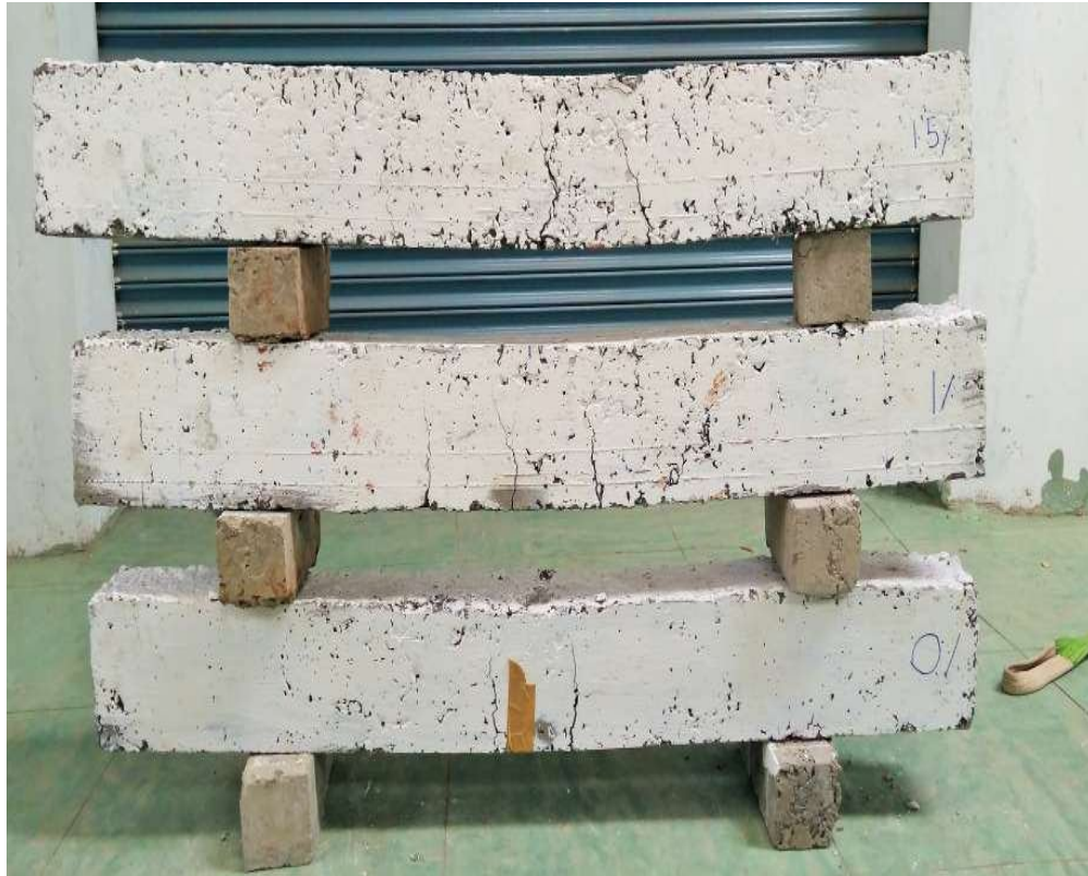
Fig 18 – Crack pattern of GPC beams with 0 %, 0.5% and 1% of glass fibres
