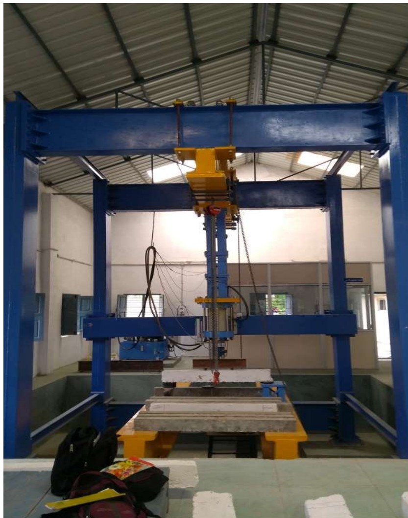
Fig 3 – Test setup for two point static loading
