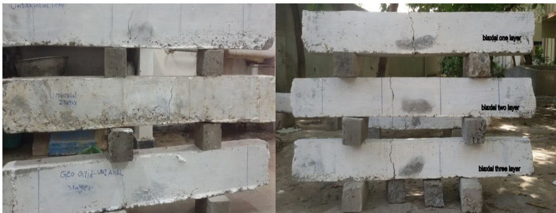
Figure.18 Beams Reinforced with Uniaxial Geogrid Figure.19 Beams Reinforced with Biaxial Geogrid
