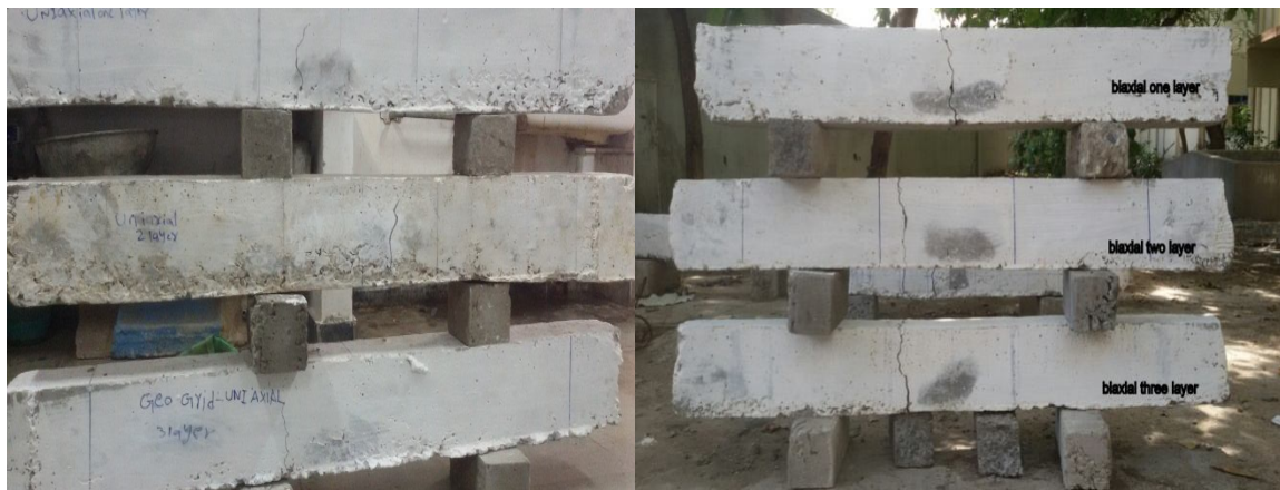
Figure.18 Beams Reinforced with Uniaxial Geogrids Figure.19 Beams Reinforced with Biaxial Geogrid
