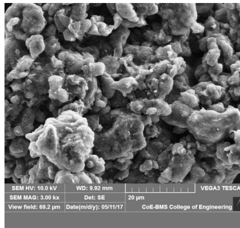
Fig 9 : SEM image of Ni coated MWCNTs
