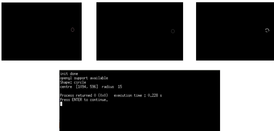
Fig. 4 Shape: Circle; a. The isolated shape after ROI extraction from source image; b. Gray smoothed image; c. Image after canny edge detection; d. Terminal showing the position of the identified vertices and the shape that it matches with.
