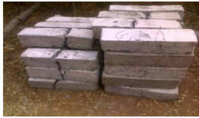
Fig 9: Stacking of tested beams
