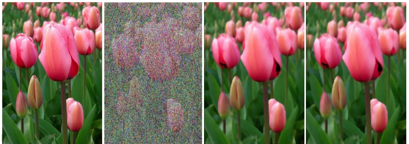
Fig.4. (a) Actual image 3 (Tulip), (b) Image contained 30% of additive impulse noise, (c) Image filtered by ANCLPVMF, (d) Image filtered PROPOSED technique.
