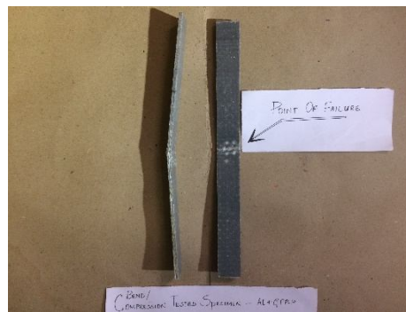
Figure.11 Sample after compression test
