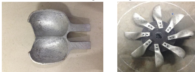
Fig. 7 Actual Pelton bucket (left) and Pelton Turbine Runner (right)
