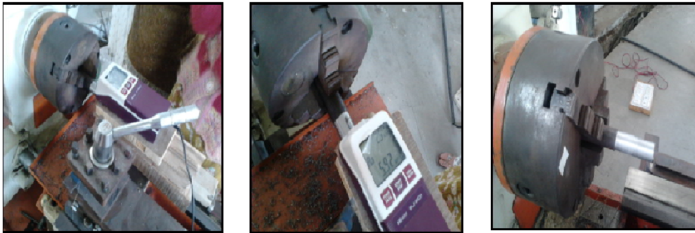
Fig. 1 Experimental details showing machining and surface roughness measurement.
