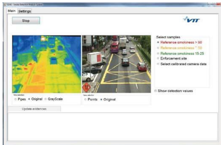
Figure 1. User interface for smoke detection and analysis system.
