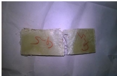
Figure 4: Glass flakes added specimen composite
