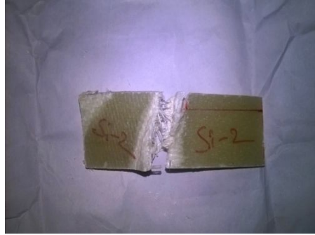
Figure 3: Silica Particles added specimen composite
