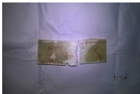
Figure 2: Pure specimen composite
