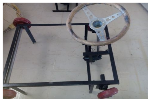
Fabrication of electrical steering mechanism
