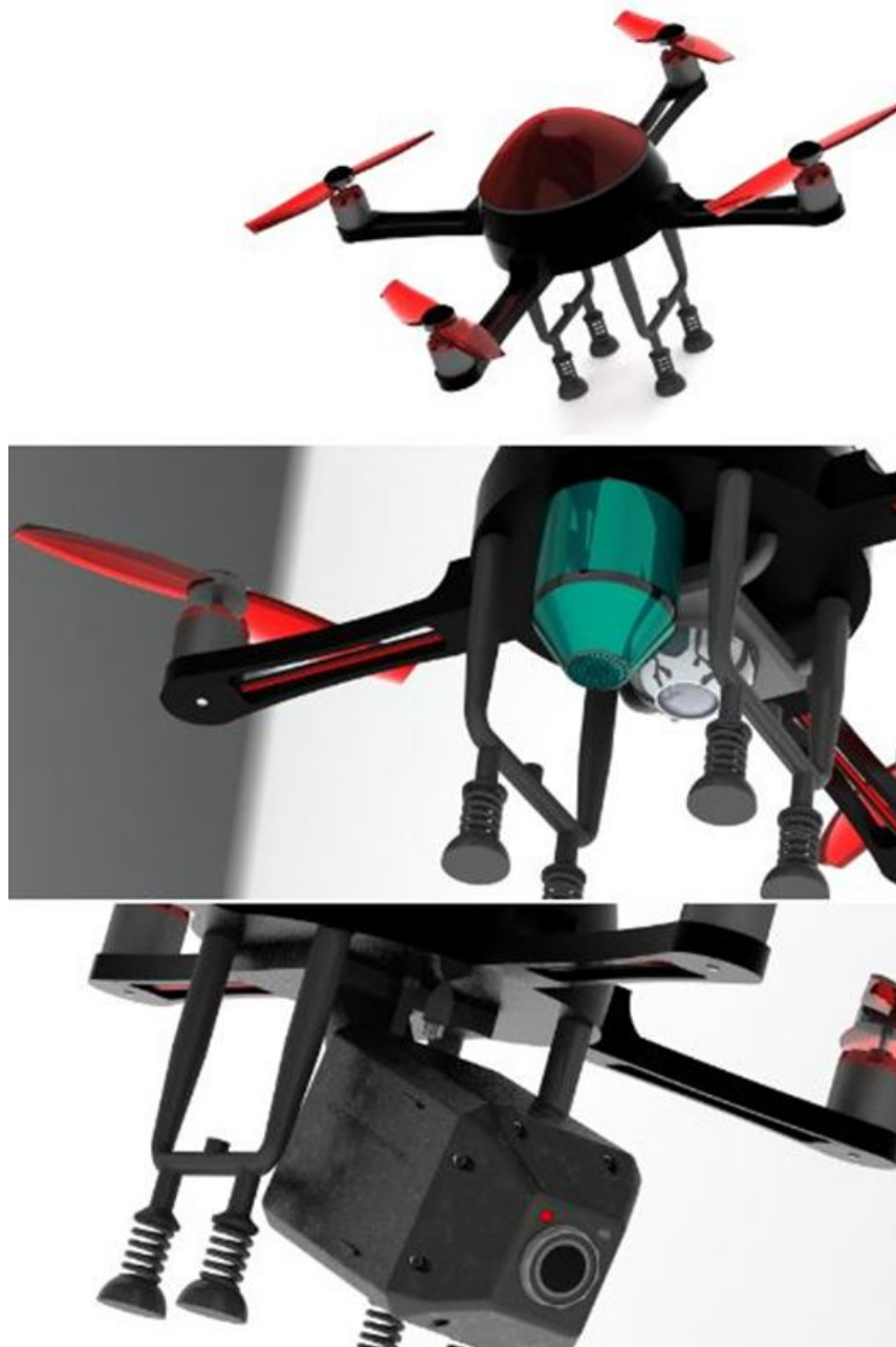
Fig 2. Modular Configuration Design Render. The Complete set of module designs is available on https://bmscemodularuav.weebly.com/modular-uavs.html
