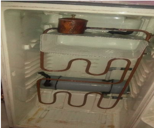
Fig. 1 Thermosyphon assisted domestic refrigerator Fig 2: Schematic diagram of thermosyphon
