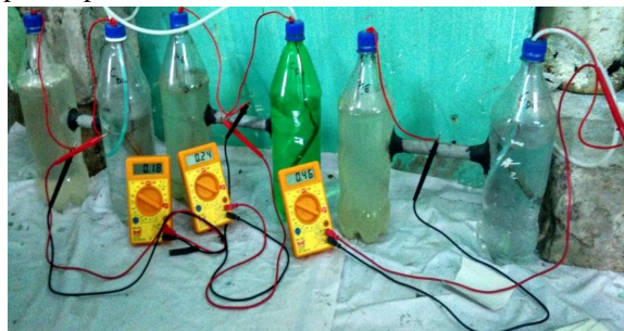
Fig. 2 Microbial Fuel Cell Setup
