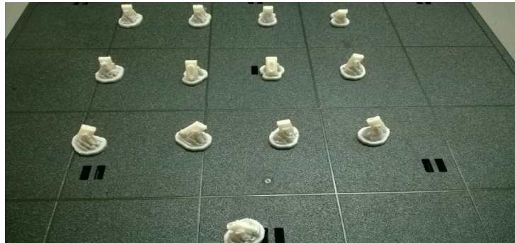
Fig: Photographic view of component printed in different orientation using FDM.
