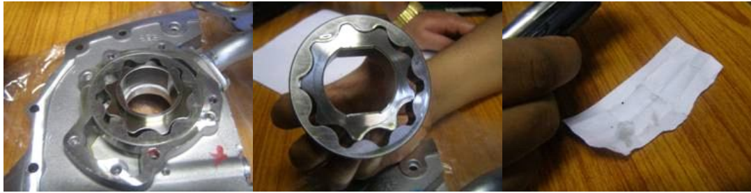
Fig-1.1: Causes of oil pump failure
