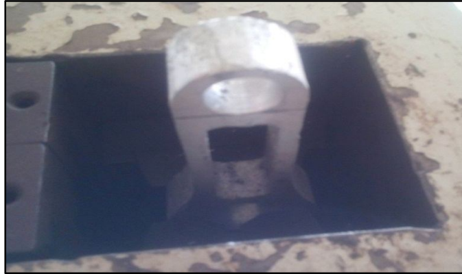
Fig:(8) Connecting rod is attached in lower jaw of Universal Testing Machine.
