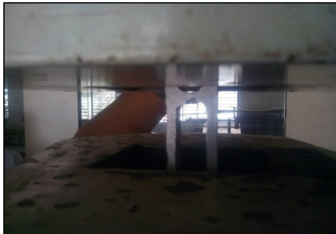
Fig: (10) connecting rod is fixed in upper and lower jaw of UTM machine.
