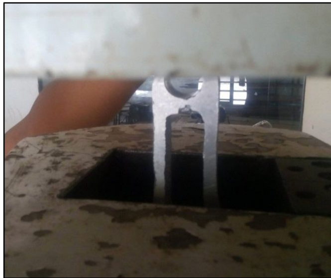
Fig: (9) After travelling lower jaw specimen is attached in to the upper jaw
