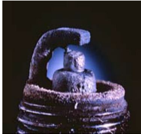
Fig. 3 Photographic view of Carbon Fouled spark plug
