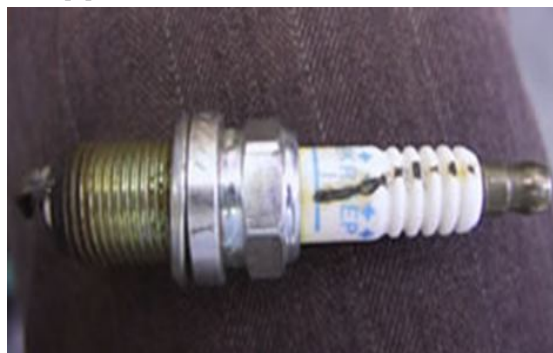
Fig. 5 Photographic view of Flash over occurred in spark plug
