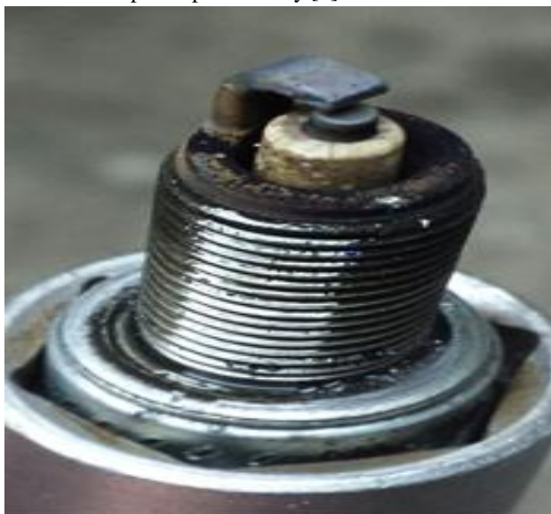
Fig. 6 Photographic view of Overheated spark plug
