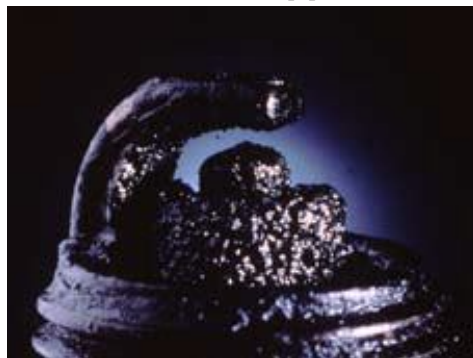
Fig. 4 Photographic view of Oil Fouled spark plug
