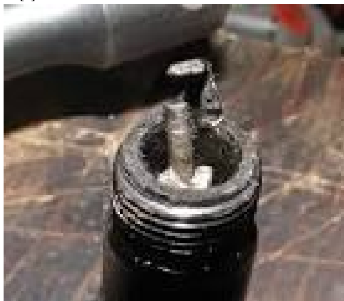
Fig. 7 Photographic view of bend of center electrode of spark plug
