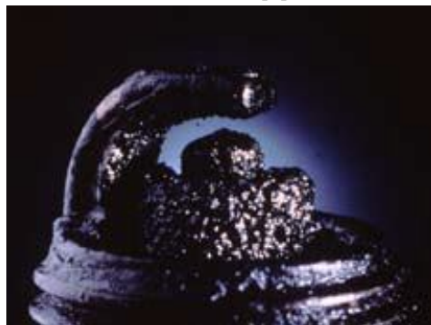
Fig. 4 Photographic view of Oil Fouled spark plug
