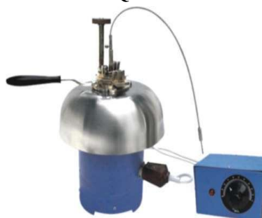
Fig. 1 Pensky – Marten Flash Point Apparatus
