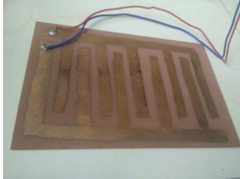
Fig.4 Copper Clad as a Sensor
