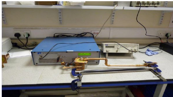
Direct Heating setup for a small scale sample
