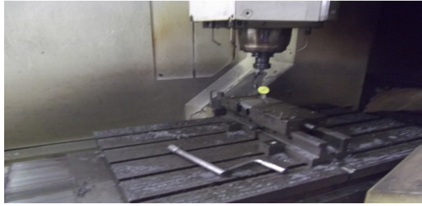
Figure 1: End Milling Operation on AISI D2 Steel
