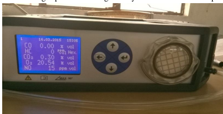
Fig.5. Exhaust gas analyzer
