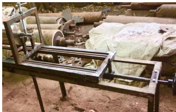
Fig 3: Guide ways for moveable clamp
