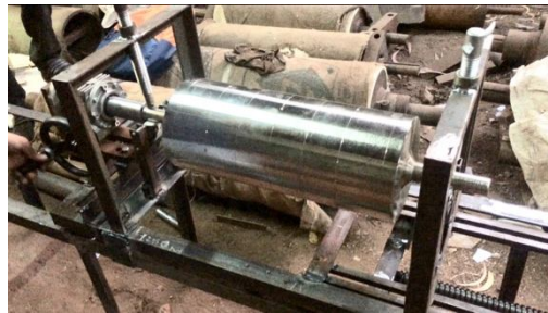
Fig 1: Workpiece mounted on clamps
