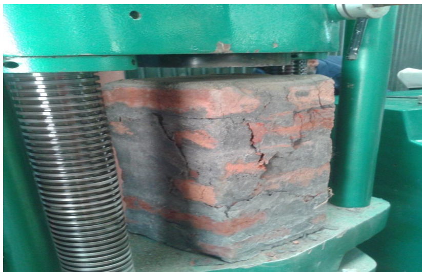
Failure pattern of sample no.3
