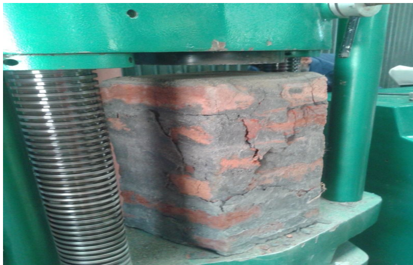
Failure pattern of sample no.3
