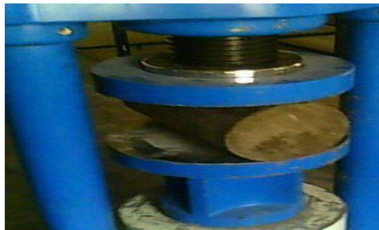
Fig 5.13 Split Tensile Strength Test with Normal Cured Specimen
