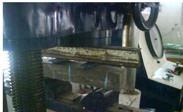
Fig 5.17 Flexural Strength with Normal Cured Specimen
