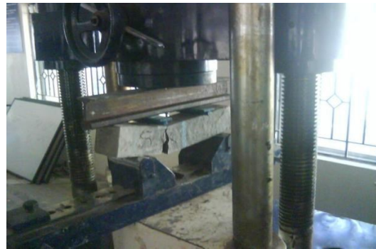
Fig 5.19 Failure Patten of Beam in Flexural Strength Test
