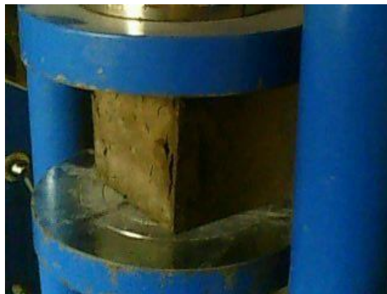
Fig 5.14 Compressive Strength Test with self cured Specimen
