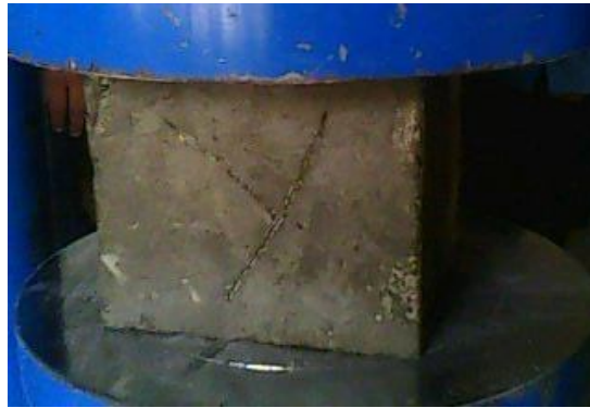
Fig. 5.12 Compressive Strength Test with Normal cured Specimen
