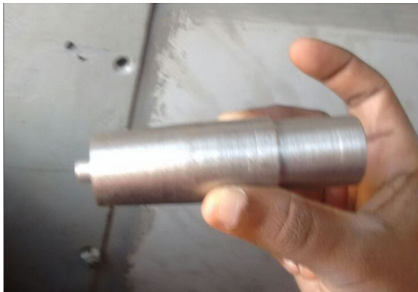
Fig 3: Tool before Nitriding, Hardness: 20 HRC.
