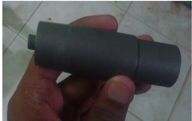
Fig 4: Tool after Nitriding, Hardness: 45 HRC
