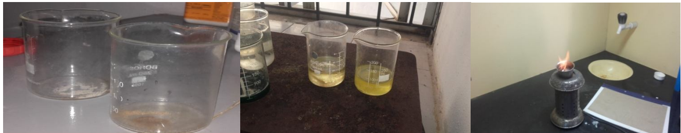
Fig4: Conventional and Used Foundry Sand Sample Fig5: Addition of Hydrochloric and nitric acid Fig6: Heating of sample after adding HF
