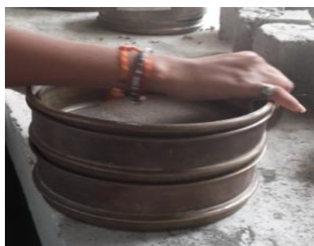
Fig7: Sieve analysis Test
