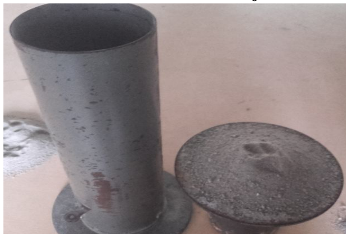
Fig10: Bulk Density Test on Conventional and Used Foundry Sand
