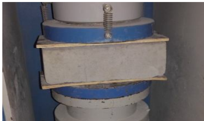
Fig12: Compressive strength test on CF and NCF Bricks
