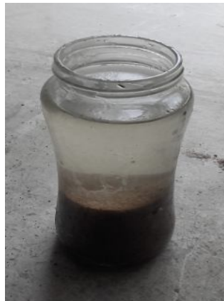
Fig8: Specific Gravity test on Conventional and Used Foundry Sand
