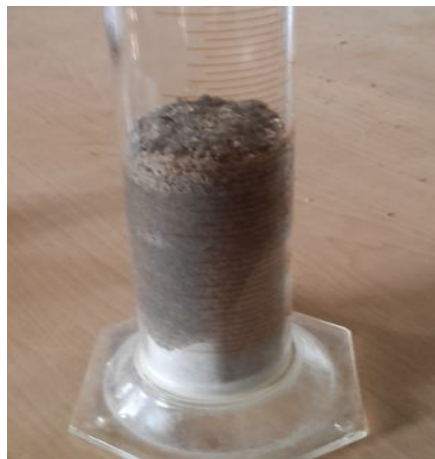
Fig9: Testing Bulking of Conventional and Used Foundry Sand
