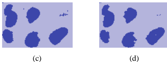
Figure 3: Segmentation results on a color image, (a) Original image (256x256x3) with gray level spread on the range [0,255]. (b) Red resulting image by FCM method. (c) Green resulting image by FCM method. (d) Blue resulting image by FCM method.
