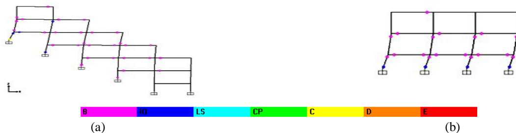
Fig 17. Hinge pattern of Type B configuration: (a) Along X-Direction; (b) Along Y-Direction
