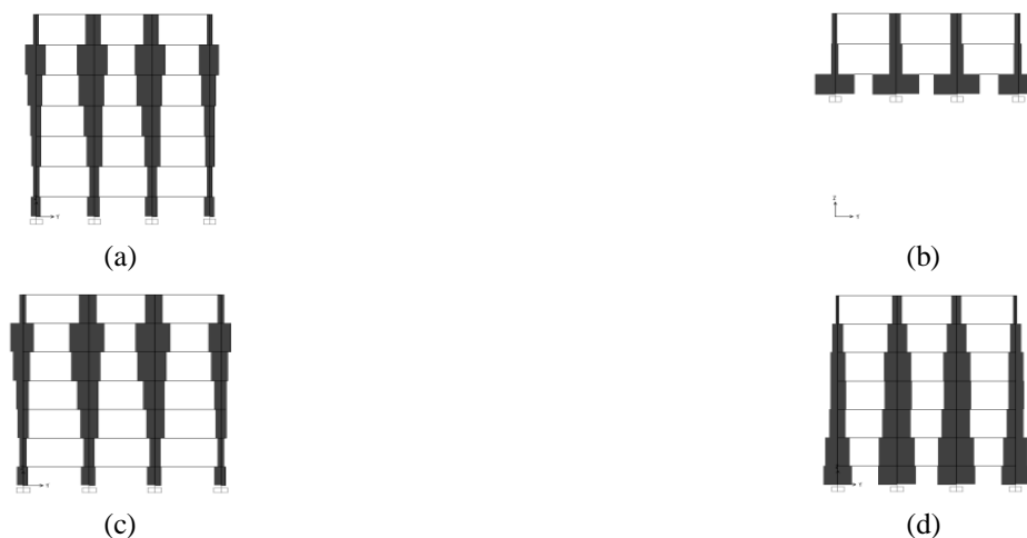
Fig 15. Variation of column shear along the height of the building due to excitation along Y-direction: (a) Type A; (b) Type B; (c) Type C; (d) Type D configuration
