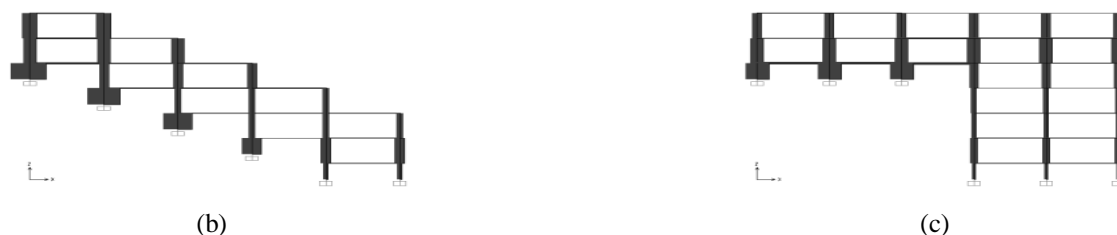
Fig 14. Variation of torsional force along height of the building due to excitation along Y- direction: (a) Type A; (b) Type B; (c) Type C
