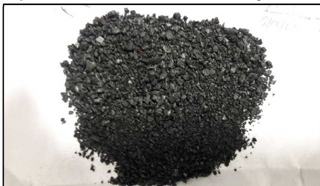
Figure 1: Prepared Charcoal from Cashew-nut shell
