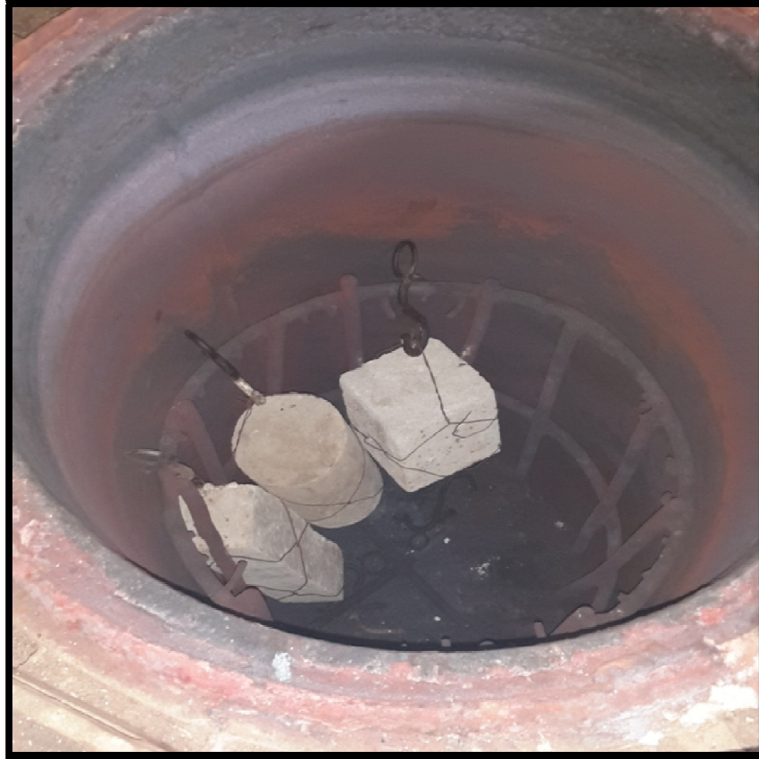
Figure 4. Concrete samples inside annealing furnace
