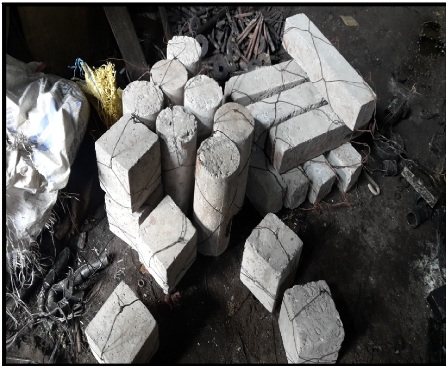
Figure 5. Concrete samples after fire test (400 o C and 800 o C)
