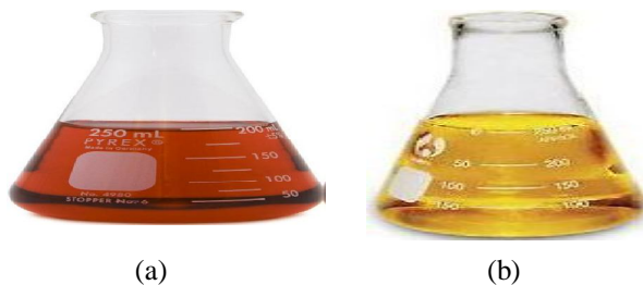
Figure 4: Sample of filtered Waste Cooking Oil (a) and the Pyrolysis biodiesel (b)
