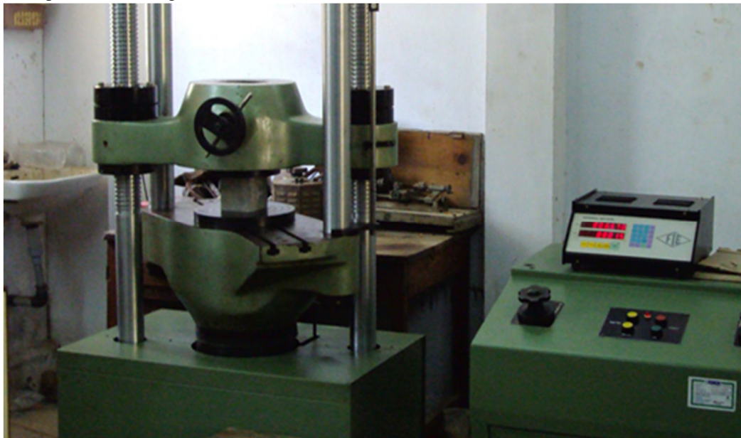
Fig. 3 Compression test in progress
