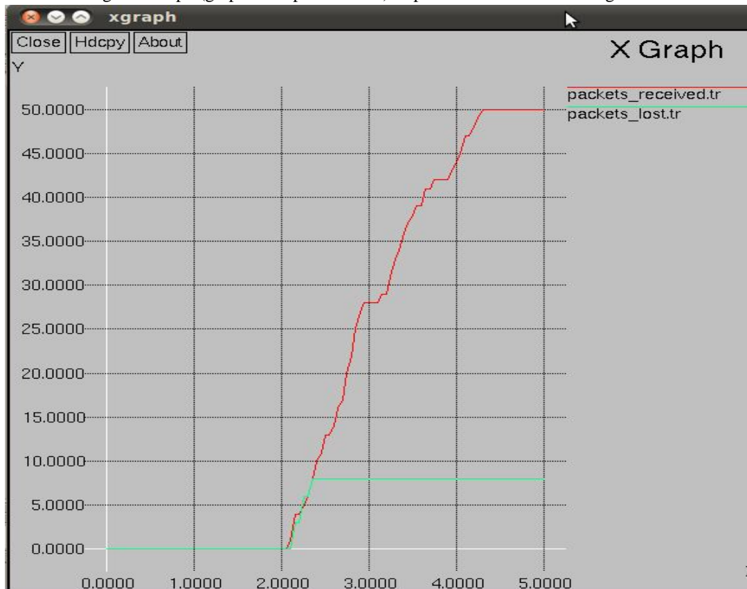
Fig 6 X Graph (graphical representation) of packets for 30 Nodes using Multi Cluster-AODV
