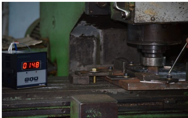
Fig. 2 Friction stir welding experimental setup with provision to measure temperatures using thermocouples
