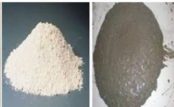
Fig 2. A Pile of Metakaolin and Spread of concrete
