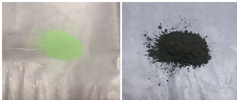
A B NiO nanoparticles (A) Before calcination and (B) After calcination
