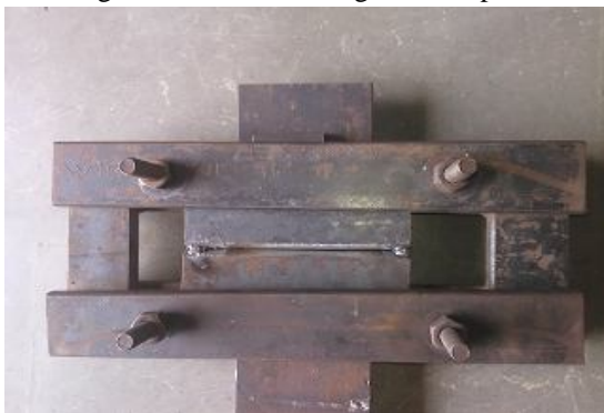
Fig. 3 Mounting of plate in fixture
