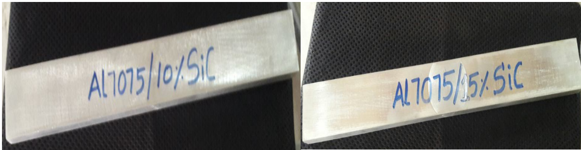
Fig 2. Al 7075-SiC(10% and15%) after casting
