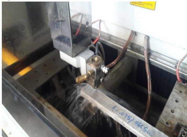
Fig1. Wire cut Electro Discharge Machine
