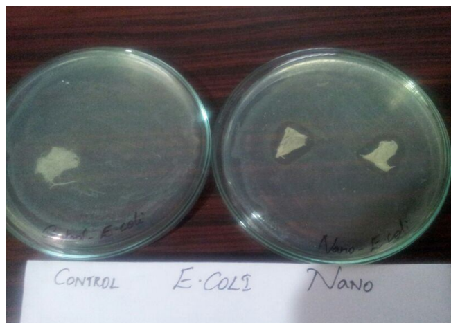
Figure 9 Antibacterial activity of cotton fabriccoated with nanoparticles synthesized using coriander extract, against E.coli
